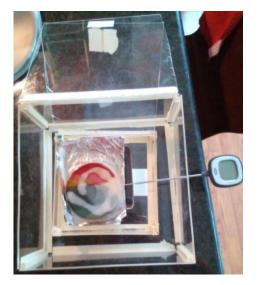
The Thrown Away Insulation will be tested in the new testing box (See side picture). The Thrown Away Insulation will be put in between the two boxes and then closed with the lid of the larger box. The testing box is made out of plexiglass.
